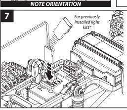
Plug the Y-harness into an open ACC port on the electronic control module (ECM). The LED lights will turn on when the ECM is powered on by plugging in the battery.
